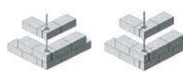
JOINT DETAILS WITH THE VERTICAL REINFORCEMENT AT CORNER OF CONCRETE BLOCK MASONRY WALLS
