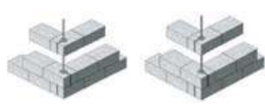
JOINT DETAILS WITH THE VERTICAL REINFORCEMENT AT CORNER OF CONCRETE BLOCK MASONRY WALLS
