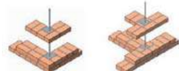
JOINT DETAILS WITH THE VERTICAL REINFORCEMENT AT CORNER OF BRICK MASONRY WALLS
