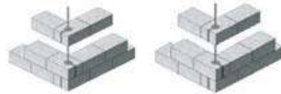
JOINT DETAILS WITH THE VERTICAL REINFORCEMENT AT CORNER OF CONCRETE BLOCK MASONRY WALLS
